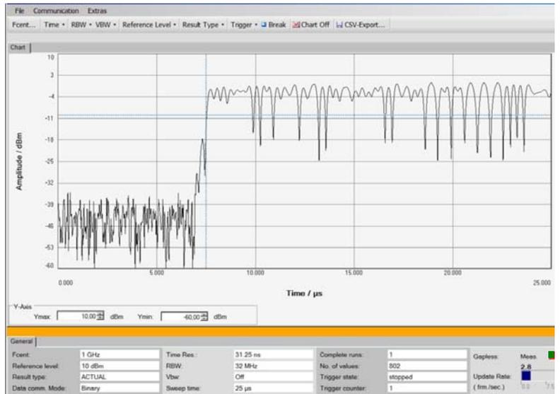
**Figure 10: Rising edge of a TDMA signal (rising edge duration approx.  $0.5 \mu\text{s}$ , frequency 1 GHz, symbol rate 3 Msym/s)**
