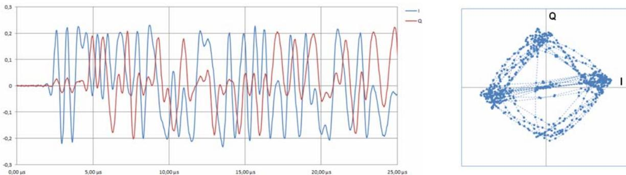
**Figure 11: TDMA signal displayed as a complex voltage with I and Q components and as a “constellation diagram”.**
