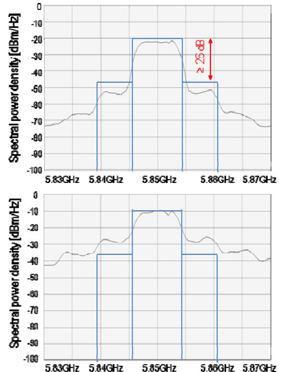
**Figure 4 top: The required sideband offset is met in this case.**
