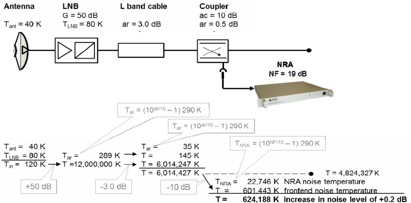
Figure 3: Determining the noise temperature
