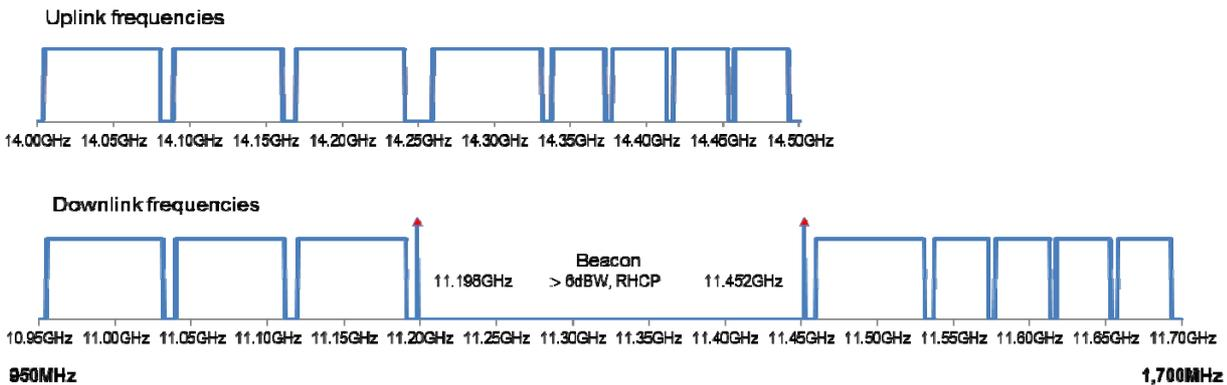
**Figure 2: INTELSAT IX spot beam frequency plan**
