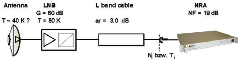
$$T_1 = G/a_r \cdot (T_{Ant} + T_{LNB}) + T_{NRA}$$
