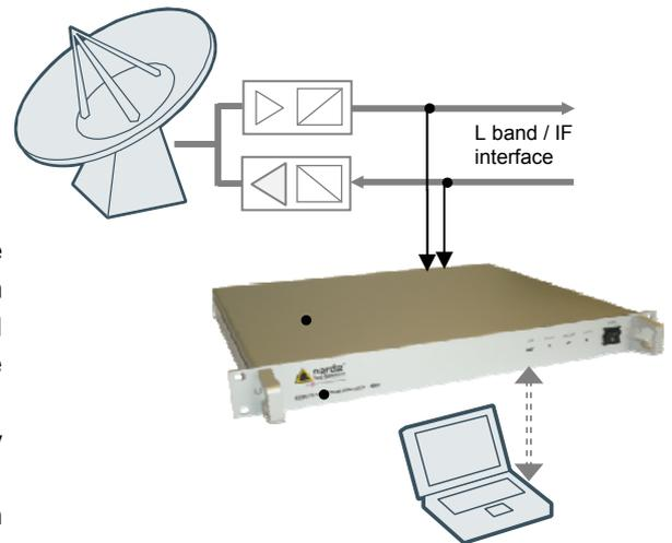
**Figure 1: Typical connection configuration in the L band / IF section of the receiving or transmitting path, with changeover switch if necessary**
