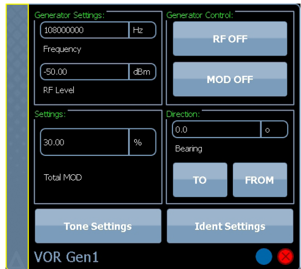
VOR Gen - Provides control of 30 Hz Var/Ref and 9960 Hz tone frequencies, modulation depths, 9960 Hz deviation, VOR bearing, to/from and ident settings.
