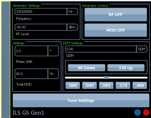
ILS Glide Slope Gen - Provides control of 90 Hz and 150 Hz tone frequencies, modulation depths, up/down DDM.
