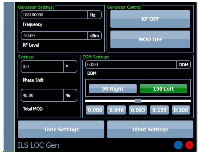
ILS/LOC Gen - Provides control of 90 Hz and 150 Hz tone frequencies, modulation depths, left/right DDM and ident settings, including Morse code.
