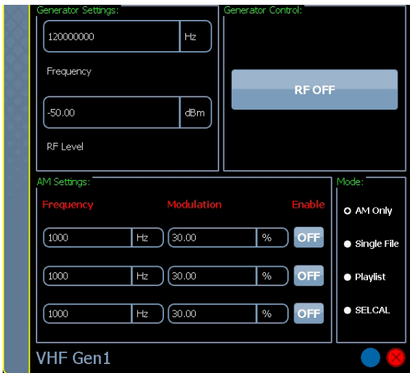
VHF Gen - Provides control of modulation frequency, modulation depth (up to 3 sources), SELCAL tones, frequency and tone sequences.
