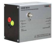
CISPR 16-2-1's most recent edition 3.0 specifies a new test method which allows the use of a coupling / decoupling network for emission measurement (CDNE) to measure disturbance voltages in the 30 to 300 MHz frequency range. This method enables EUTs to be connected directly to the CDNE, allowing a single conducted emission measurement to replace a lengthy radiated emission test. Product standards may use this fast, convenient and economical alternative.
