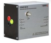
The publication of EN 55015, based on CISPR 15 A1 Ed.7, has introduced an independent method of measurement of radio disturbance characteristics of electrical lighting equipment. This method specifies the use of a coupling/decoupling network (CDN) as defined in IEC 61000-4-6 for emission measurement in the frequency range 30 MHz to 300 MHz.
