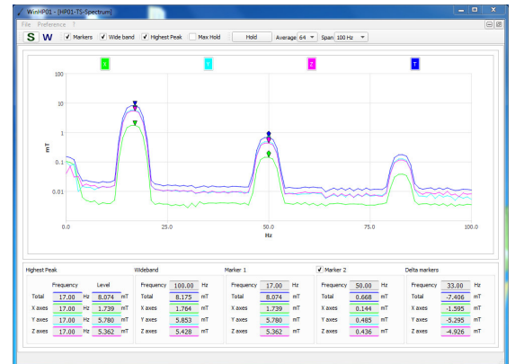
Figure 6: FFT analysis with display of amplitude spectrum
