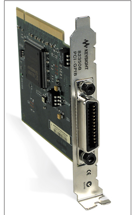
82350B PCI high-performance GPIB interface card
