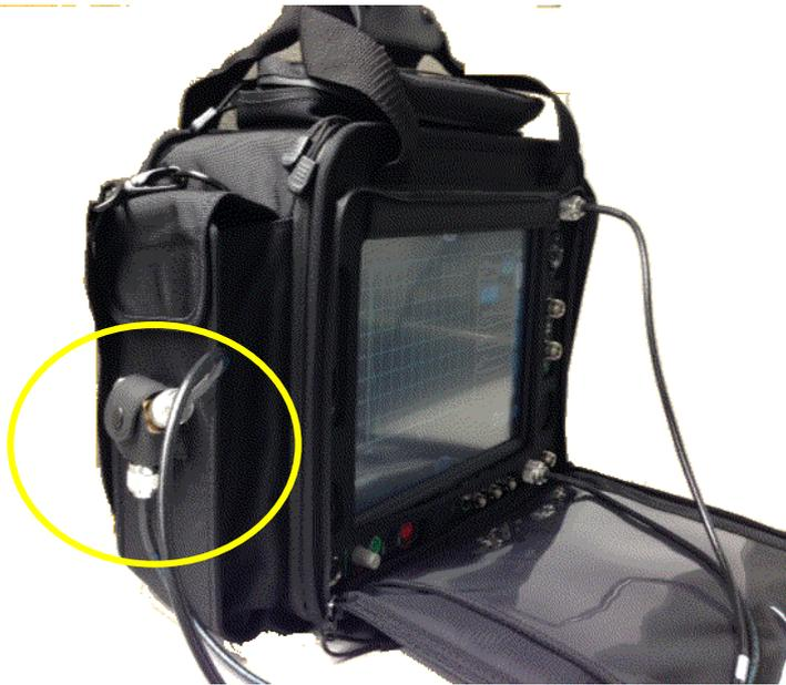
With the optional Soft-Sided Carrying Case, the Power Divider can be mounted for quick and easy access. Simply connect the provided N Type cables from the 8800S to the Power Divider.
