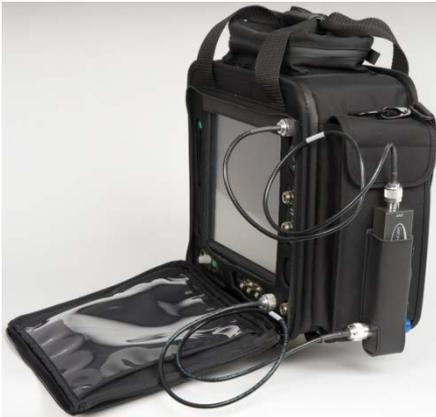
With the optional Soft-Sided Carrying Case, the Return Loss Bridge can be mounted for quick and easy access. Simply connect the provided N Type cables from the 8800S to the Return Loss Bridge.
