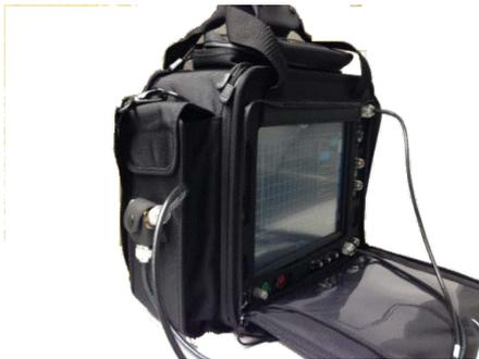
With the Return Loss Bridge you can measure Antenna or Device Return Loss or VSWR.
