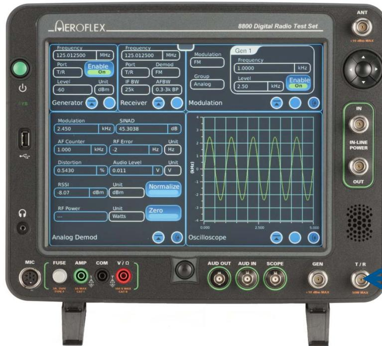
For basic Transmitter and Receiver tests, connect the 8800S TR port to the Radio ANT port.
