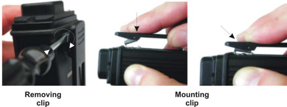
Figure 2 -Clip installation/removal
