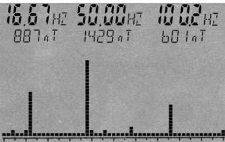
LF spectrum display and automatic multi-marker display on the digital screen of SPECTRAN® (Screenshot)
